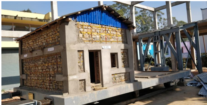
Figure 2: Test setup showing impact hammer (right) and strengthened model.
