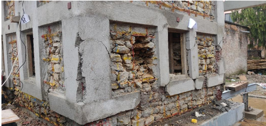
Figure 7: Impact aided damage to the specimen.
