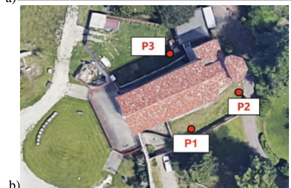
Figure 2. a) The principal investigations previously performed; b) location of the monitoring boreholes equipped with extensometers and optical fiber cables.
