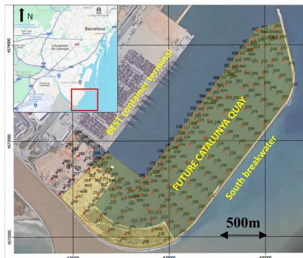
Figure 1. Geotechnical site investigation of the future Catalunya quay, 2022-2023. Points: red (boreholes), blue (CPTu) and green (SDMT).
