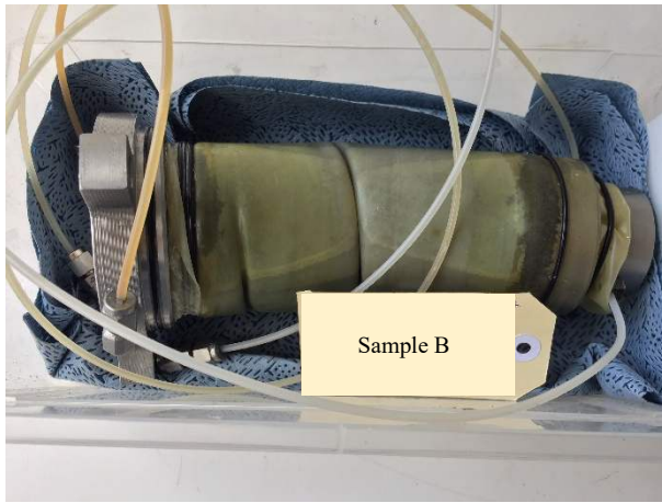
Figure 4. End of RCA test soil sample: as placed in the freezer
