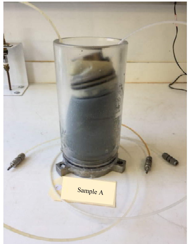
Figure 3 End of RCA test soil sample: fully liquefied, isolated with quick-release connection fittings
