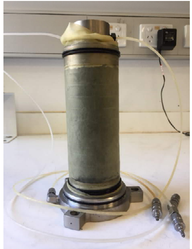
Figure 2. Soil sample prepared by moist tamping within the new RCA modular set-up
