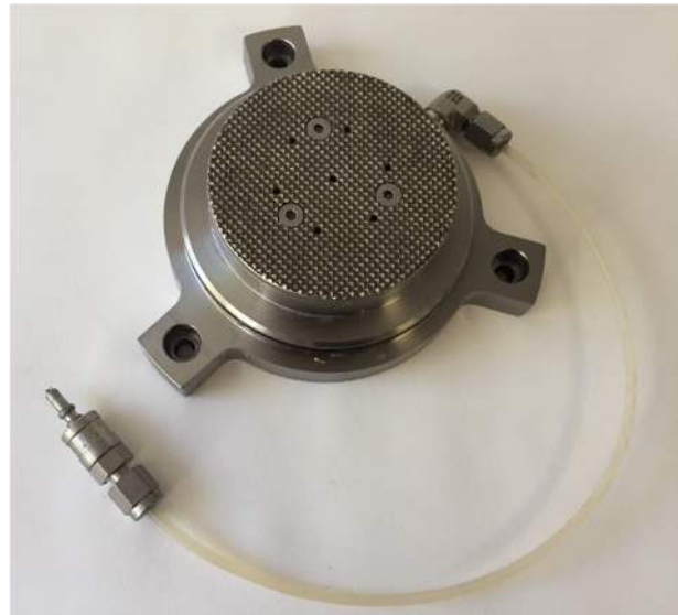
Figure 1. New modular base platen for the RCA apparatus
