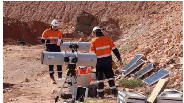
Figure 4. Two muon detector telescopes mid-installation (note not their final placements), with the background muon counter as the small black box at its base.
