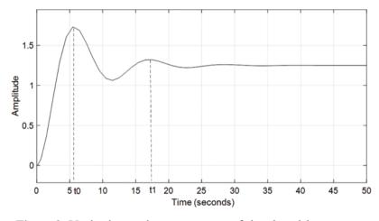
Figure 3: Underdamped step response of the closed-loop system
