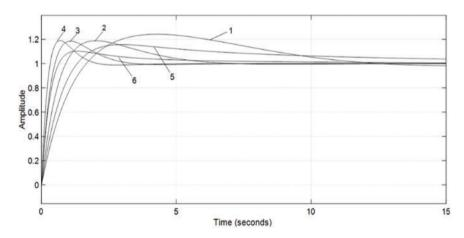
Figure 5: Transient responses of the automatic control system
