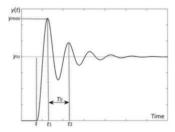
Figure 2: Underdamped step response of the closed-loop system
