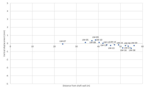
**Figure 9.** Ground Surface Levelling around the Electrical Tower during Diaphragm Wall Installation
