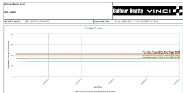
**Figure 12.** Contractor’s monitoring system “Mission OS” data platform output for the week from 18th September to 22nd September 2023, when the excavation reached 43m AOD.
