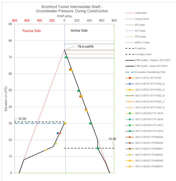
**Figure 13.** Groundwater pressure measured by the different vibrating wire piezometer tips after the excavation reached formation level, indicated by the horizontal blue dashed line on the passive side (excavation side). On the active side (ground side) the groundwater pressure profile indicated by tunnel alignment piezometers together with the shaft piezometer 1MC13.BTIS167-PV-601, located at the outside of the diaphragm wall perimeter.
