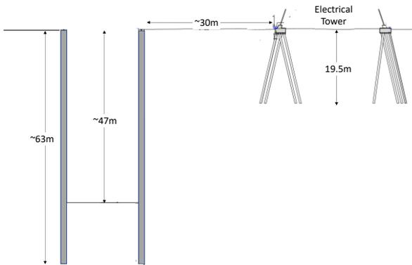
**Figure 6.** Section Through Shaft Illustrating Interface with the Electrical Tower
