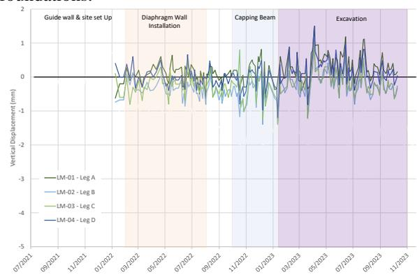
**Figure 8.** Levelling of Electrical Tower Bases
