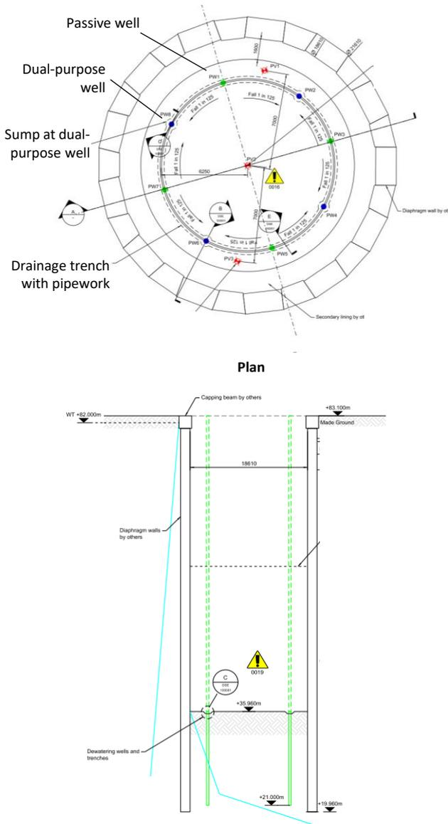
**Figure 4.** Depressurisation System showing Design Pore Pressure at Formation Level
