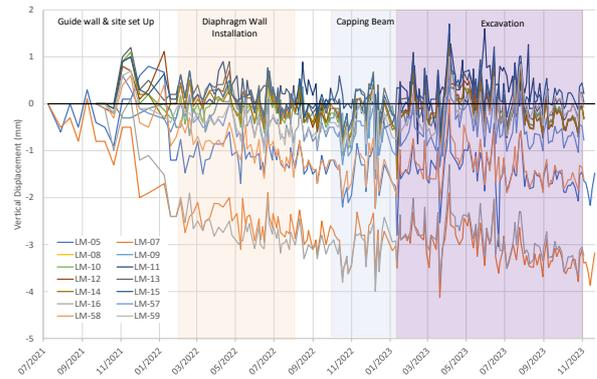
**Figure 7.** Ground Surface Levelling Around the Electrical Tower
