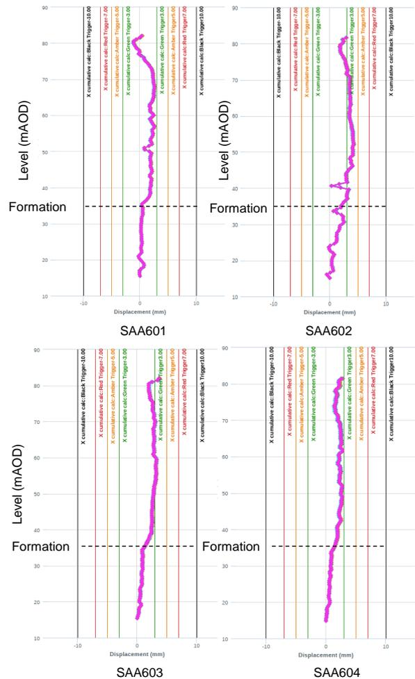
**Figure 11.** SAA Measured Diaphragm Wall Movement at the end of Shaft Excavation
