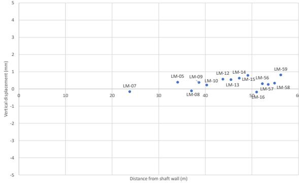
**Figure 10.** Ground Surface Levelling during Shaft Excavation
