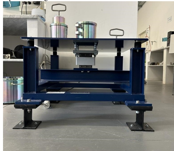
Figure 4. Apparatus for estimating e_{max} and e_{min} at the Soil Dynamics and Geotechnical Engineering Laboratory of the University “Kore” of Enna (Italy).
