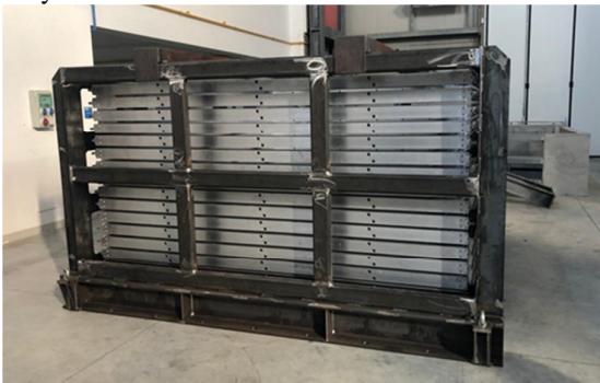
Figure 1. Laminar shear box at L.E.D.A. of the University of Enna “Kore”.
