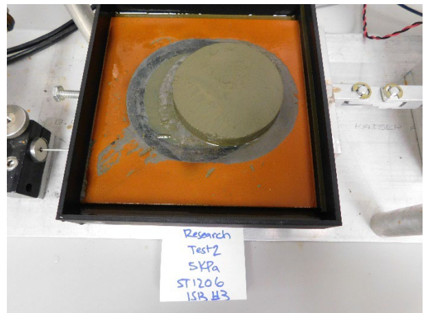
Figure 8. Adhesion on the clay specimen to the steel interface plate during shearing
