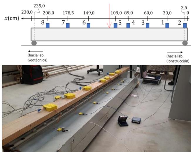
Figure 10: Location of the sensors – Stringer beam test
