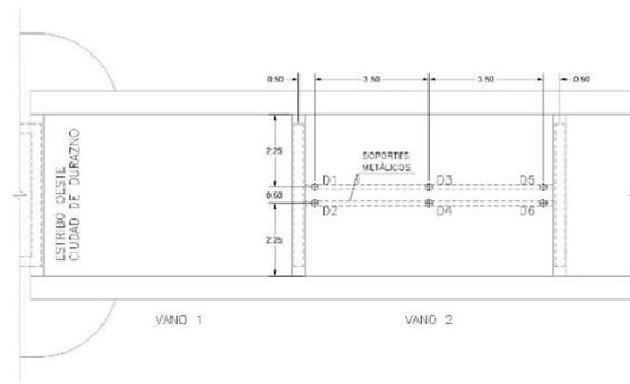
Figure 5: Plan view. Displacement sensors location.
