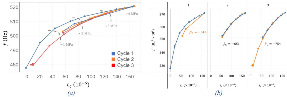
Figure 2: (a) Fundamental torsional frequency of vibration with respect to compressive strain, and (b) squared fundamental torsional frequency with respect to compressive strain.
