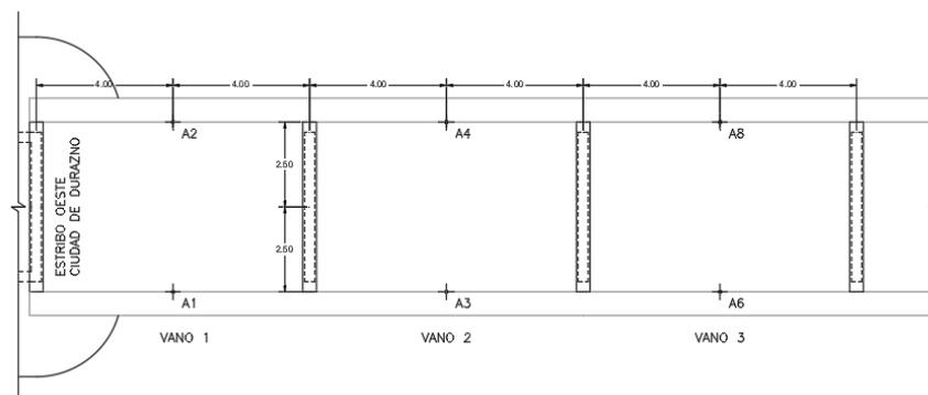
Figure 6: Disposition of sensors during Structural Health Monitoring stage.
