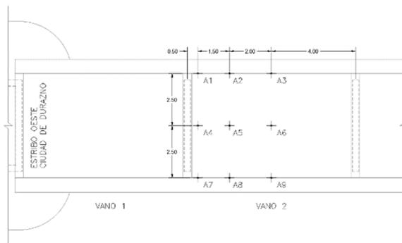
Figure 4: Plan view. Accelerometers location.
