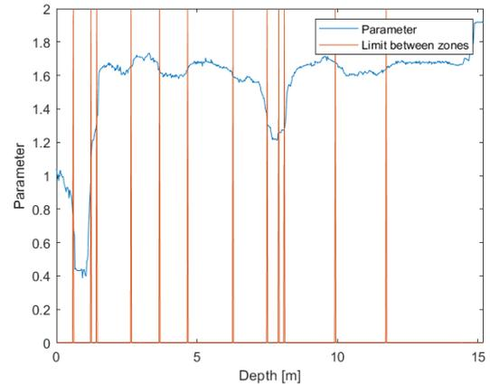
**Figure 11.** Alteration index and subdivisions determined by Amokrane's algorithm for survey 3
