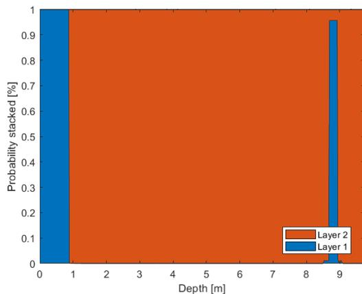
**Figure 9.** Probabilities calculated for each point in the drilling log of belong to a given soil layer for survey 2
