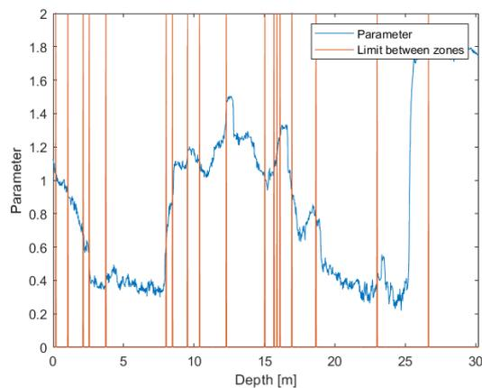
**Figure 6.** Alteration index and subdivisions determined by Amokrane's algorithm for survey 1
