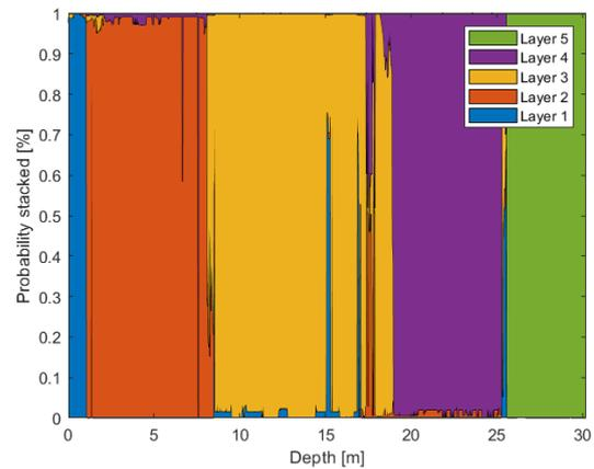
**Figure 7.** Probabilities calculated for each point in the drilling log of belong to a given soil layer for survey 1
