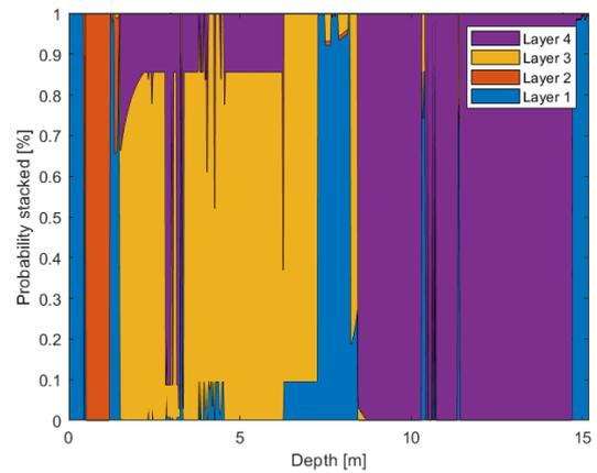
**Figure 10.** Probabilities calculated for each point in the drilling log of belong to a given soil layer for survey 3
