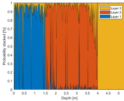
**Figure 5.** Probabilities calculated by Moussouteguy's algorithm for synthetic signal 2
