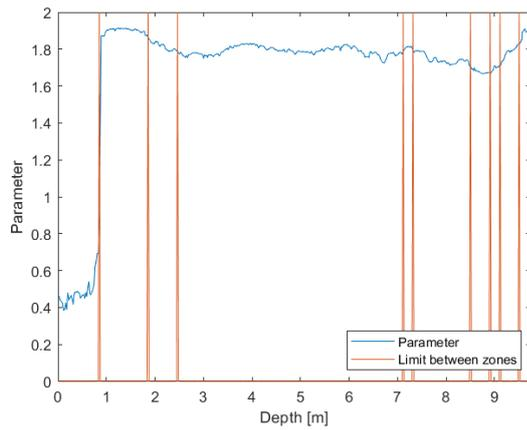
**Figure 8.** Alteration index and subdivisions determined by Amokrane's algorithm for survey 2
