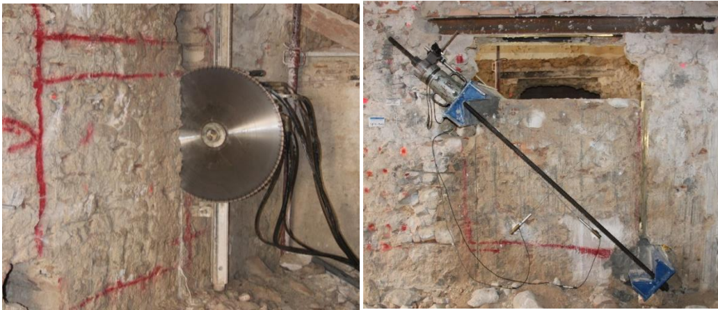
Figure 1: Left, Circular saw cutting the masonry specimen. Right, experimental equipment for the DC test.
