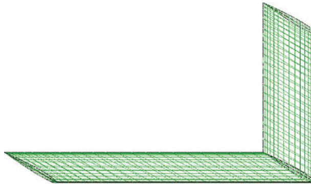
Figure A3: OpenVSP model of the Bertin-Smith wing
