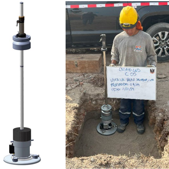
a) LWD Dynatest 3031 b) Photo of field LWD test
