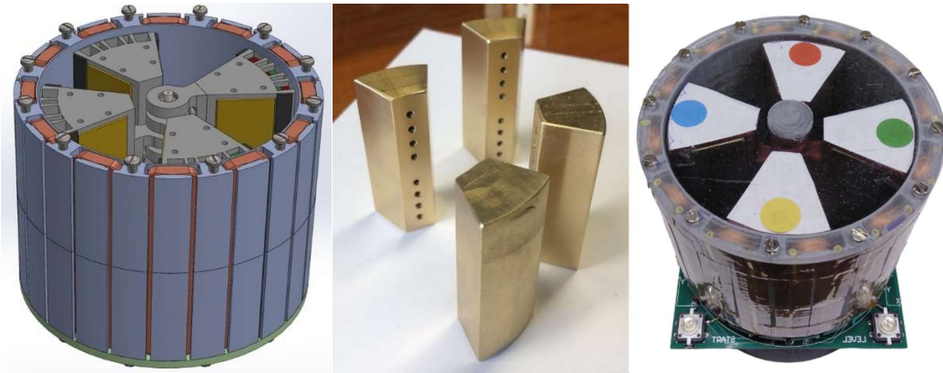
Figure 2: 3D model of the harvester (a), brass parts (b), and actual harvester (c)
