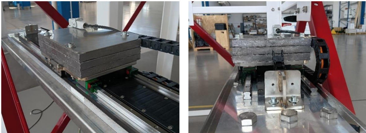
Figure 6: Picture of the 2 AMDs installed on a trellis mock-up realized in the ISAAC laboratories
