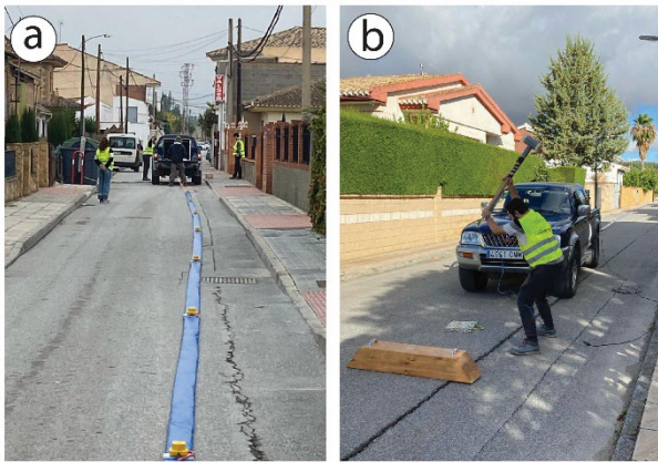
Figure 3. (a) Land-streamer, with 4.5Hz triaxial geophones, being towed through the Fuente Vaqueros streets; (b) Sledgehammer-based seismic source for generating Rayleigh (plate), and Love (wooden beam) waves.
