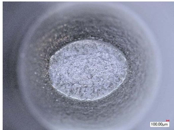
Fig. 33. Fracture surface for expanded circumferential tensile test specimen.
