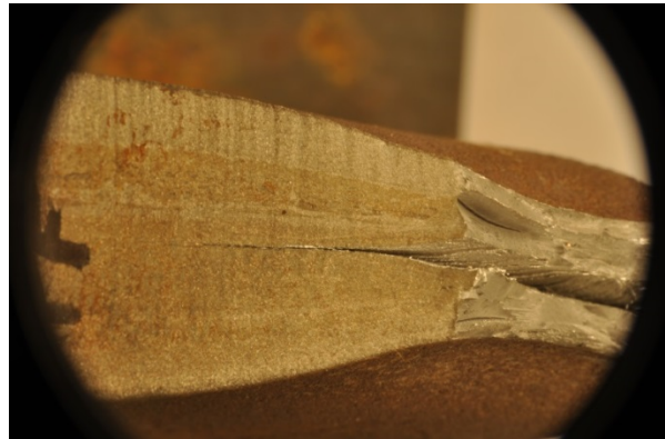
Fig. 51. Side view of fracture surface for expanded and strain-aged longitudinal tensile test specimen 90° from weld seam.
