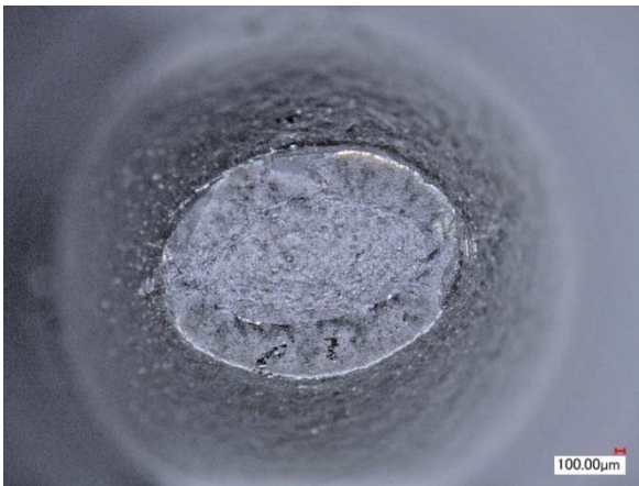
Fig. 32. Fracture surface for as-rolled circumferential tensile test specimen.
