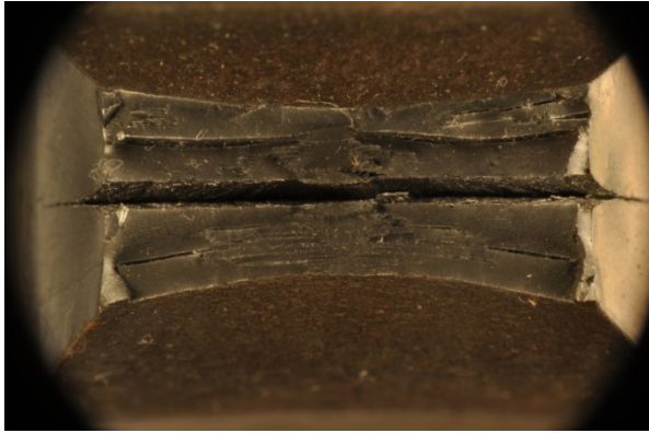
Fig. 46. Top view of fracture surface for as-rolled longitudinal tensile test specimen.
