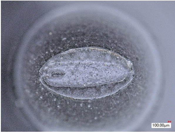
Fig. 41. Fracture surface for expanded and strain-aged longitudinal tensile test specimen 90° from weld seam.
