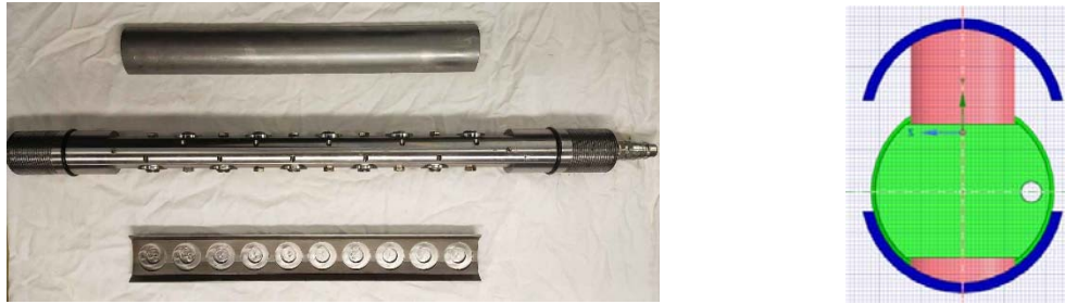
Figure 3. On the left: The Fondasol rigid dilatometer (disassembled). On the right: Schematic cross-sectional view of the probe illustrating one shell spread apart while the other remains in its initial position
