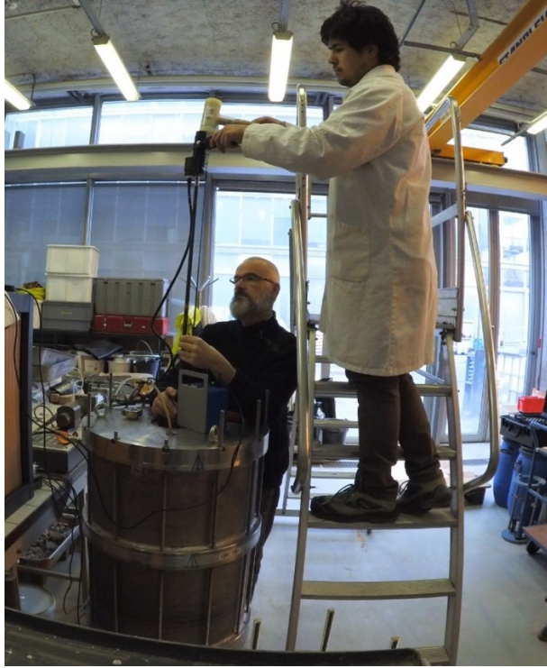
Figure 9. Dynamic penetrometer installed and dynamic driving over the specimen.
