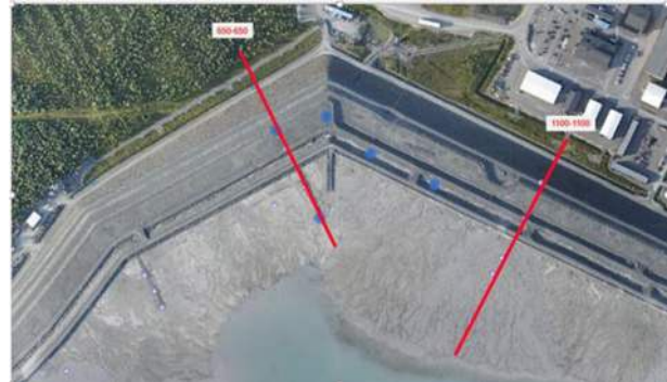
Figure 1. Intended area to be monitored is the slope of the TSF located between the two red lines (North direction is up).
