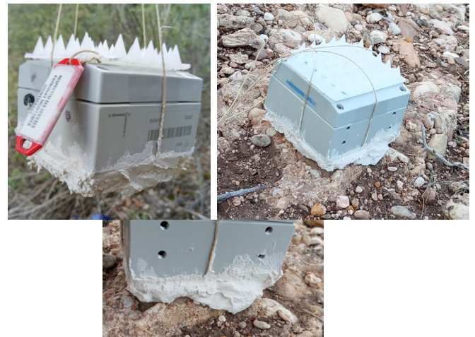
Figure 12. Close-up view of the TIL90 sensor that was installed in the 'Panxo-A' block. Left: sensor hanging from the drone, with identification label (red) and with a system to prevent birds from landing on the equipment (white spikes). Right: sensor once placed on top of the block. Bottom: detail on how, during the drop of the sensor, the perimeter cord of cement-glue (figure 5) has adapted to the irregularity of the underlying rock.
