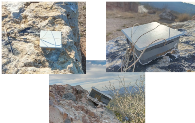
Figure 10. January 2024, first landings with dummy boxes and adhesive. The boxes were left with inclination angles of 5°, 11° and 35°, respectively.
