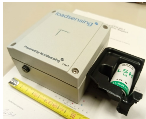
Figure 3. Worldsensing Tiltmeter TIL90-i (weight 440g). The overall box dimensions are 10cm x 10cm x 6cm. With the 3.6Volt battery (right, weight 51g) the sensor can operate several years for a reporting period of 5 minutes and average weather conditions.
