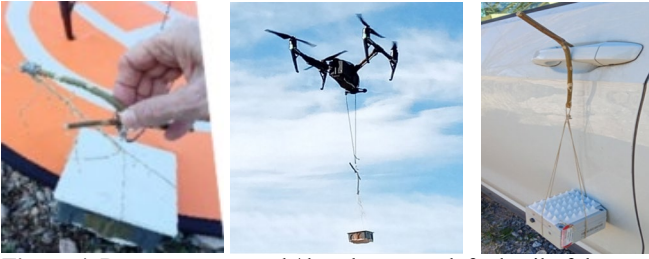
Figure 4. Drone-sensor attach/detach system: left, detail of the “Y” piece; center, sensor hanging from the drone; right, sensor, line and “Y” piece ready for attach.
