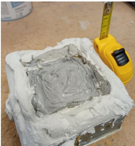
Figure 5. Adhesive layout on the lower base of the sensor.
