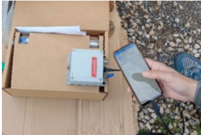
Figure 8. Initialization of an INC15 tiltmeter using an App from the mobile phone.
