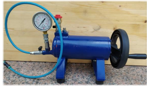
Figure 4. manual pressurization System and manometer (first prototype)
