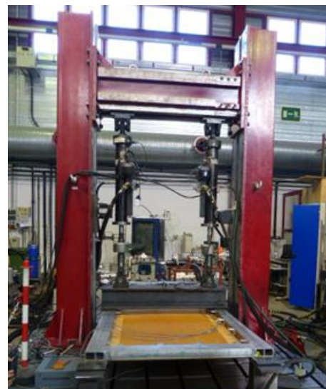
Figure 15. Bending test for the demonstrator.
