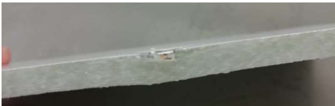
Figure 35 – Disruption of the fibres' alignment caused by the accelerometer in T2C.
