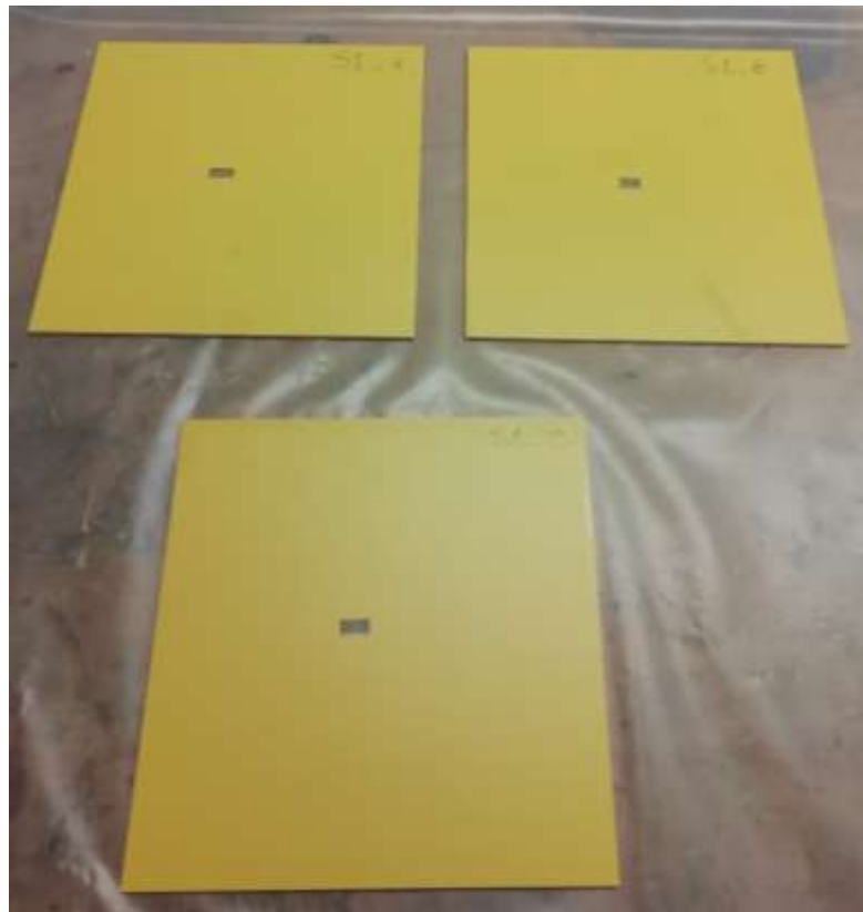
Figure 43 – S1 after cutting, resulting in S1_A, S1_B and S1_C.
