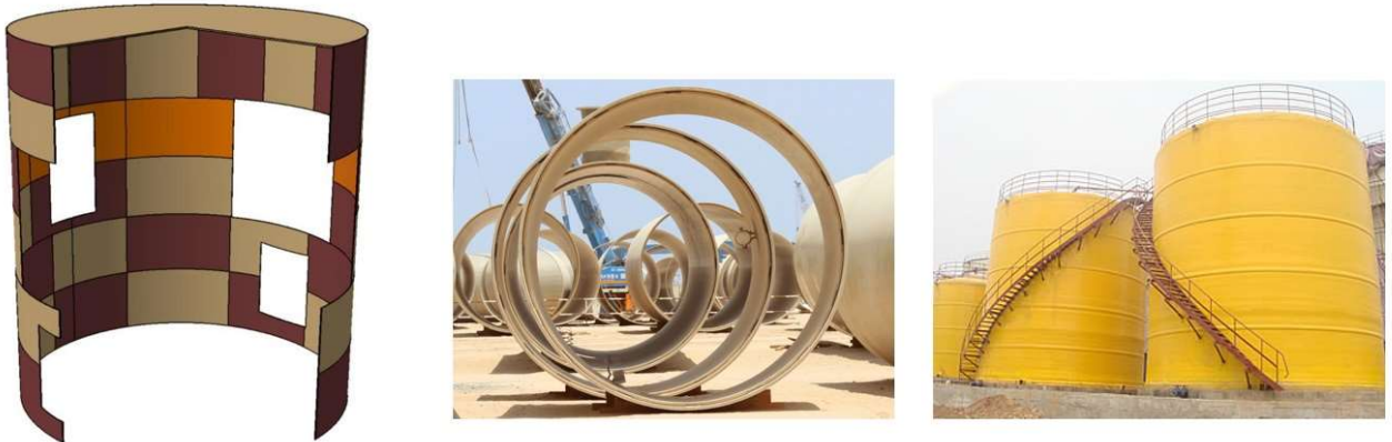
Figure 22 : main cylinder 3D and large filament winding cylinders
