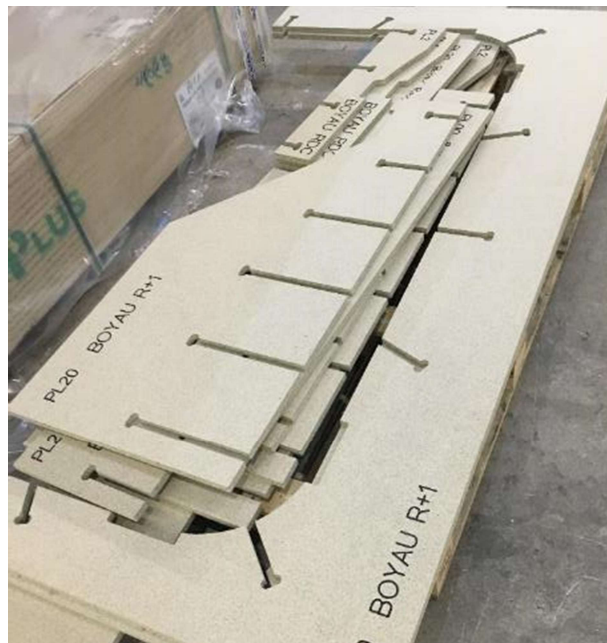
Figure 6 : Mould structural panels
