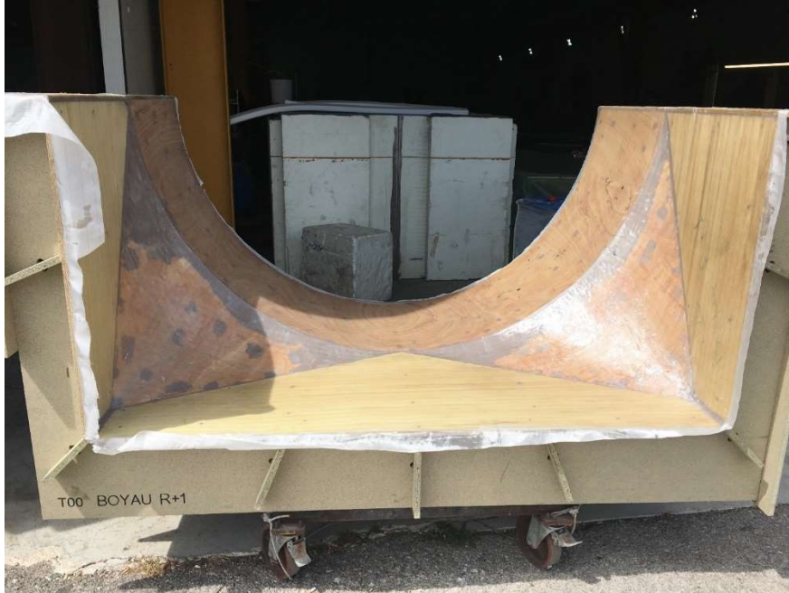
Figure 7 : Structural part of the mould
