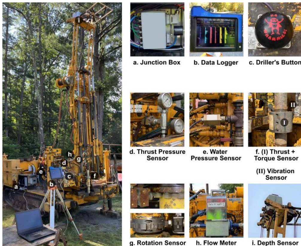
Figure 2. Measurement While Drilling equipment at the New Hampshire Department of Transportation, USA.
