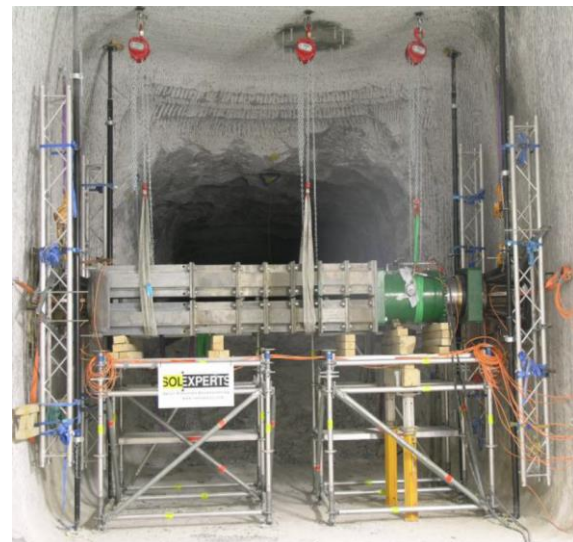
Figure 10: Example for horizontal plate load test setup showing the bearing plates, hydraulic jack (green), extension and the load support arrangement.
