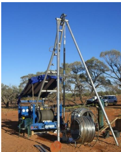
Figure 7: Lean and cost-efficient set-up for mini-HF measurements in a 2000 m deep borehole in Australia showing the double packer probe. No drill-rig and crew required.
