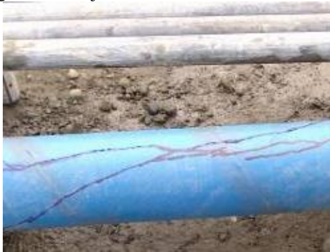
Figure 6: Impression packer for the determination of the fracture orientation.
