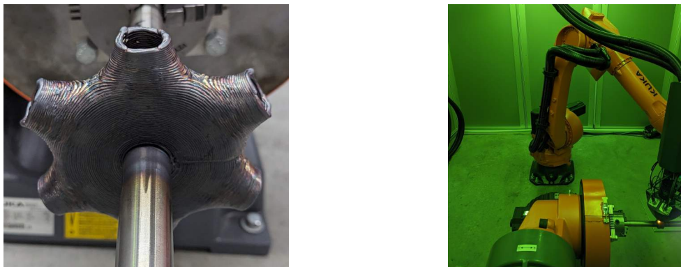
Figure 7: Left: Completed node affixed to the supporting rod and rotary table. Right: Integrated Meltio Engine, KUKA robotic arm, and rotary table during node fabrication.
