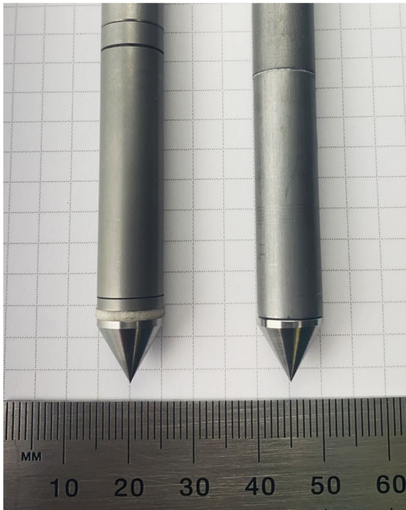
Figure 3. Miniature CPTu (left) and CPT (right) cones.
