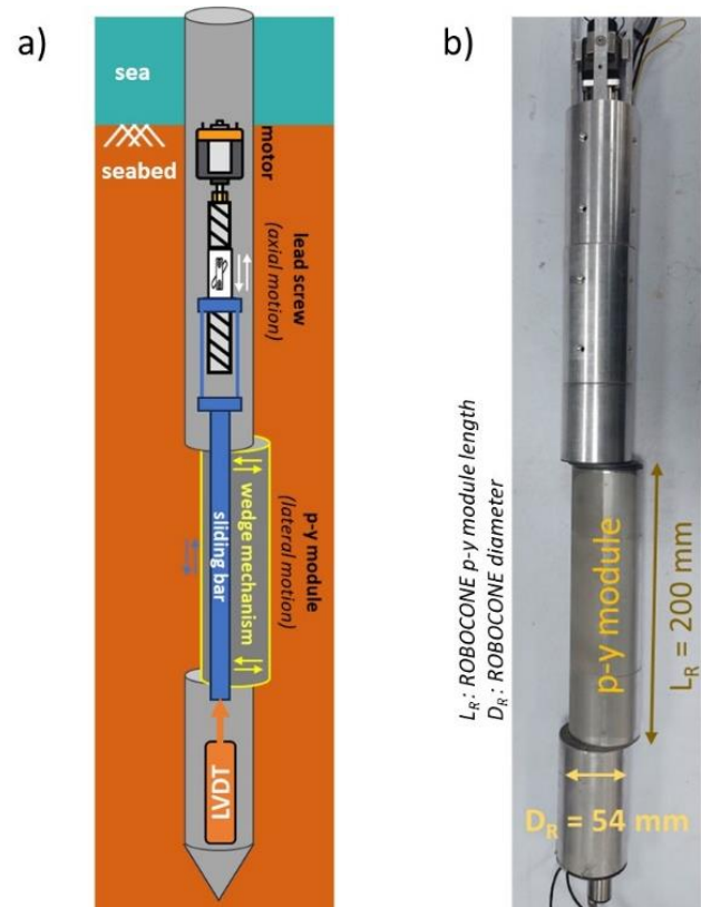
Figure 2. The ROBOCONE p-y module: (a) schematic drawing; (b) initial aluminium prototype.
