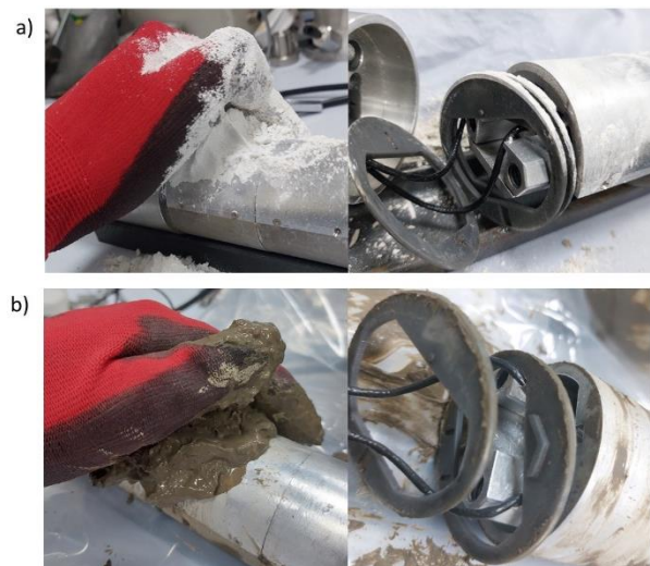
Figure 6. Sealing investigation against fine soil ingress: (a) kaolin clay powder; (b) marine clay slurry.
