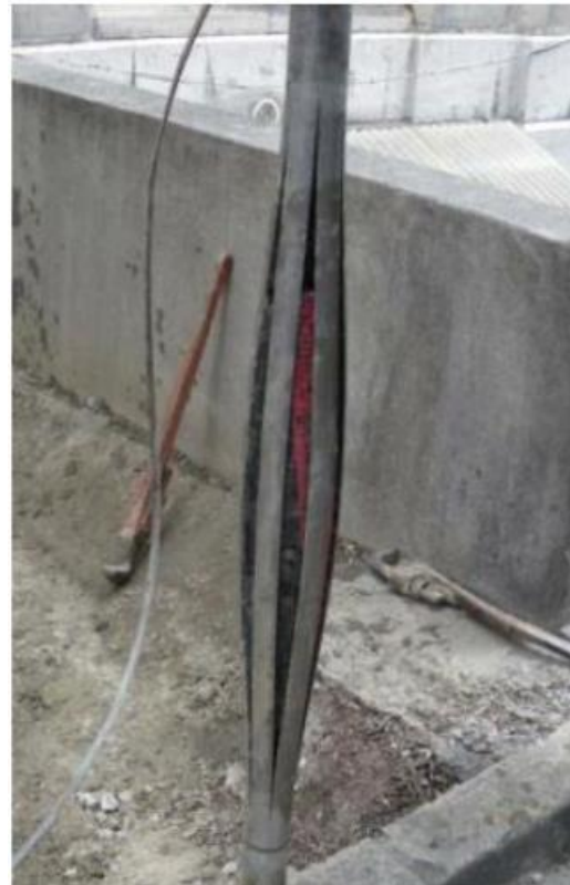
Figure 2: Deformation of the bare probe (a) and lantern probe (b) in own resistance (Monnet et al. 2022)
