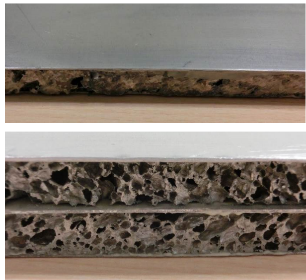
Figure 1. Examples of (top) single and (bottom) double foam core panels
