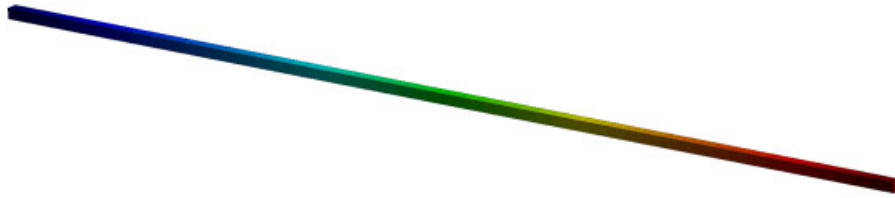
Figure 1. Norm of the displacement for the clamped beam.
