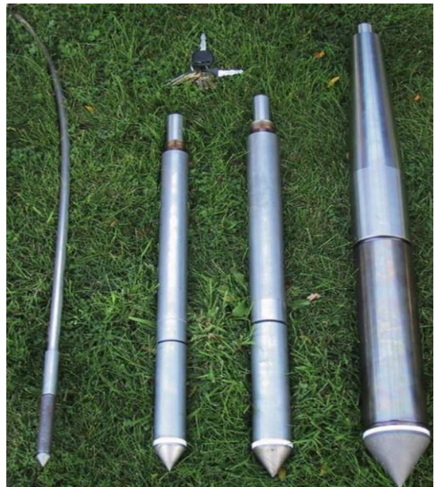
Figure 1. 5 cm 2 , 10 cm 2 , 15 cm 2 and 40 cm 2 penetrometers (Robertson and Cabal, 2012).
