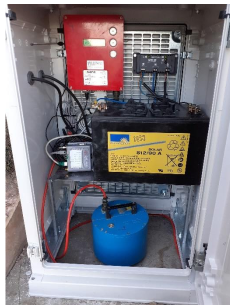
Figure 3. Monitoring equipment of each device: seismometer, recorder, power supply and communications.
