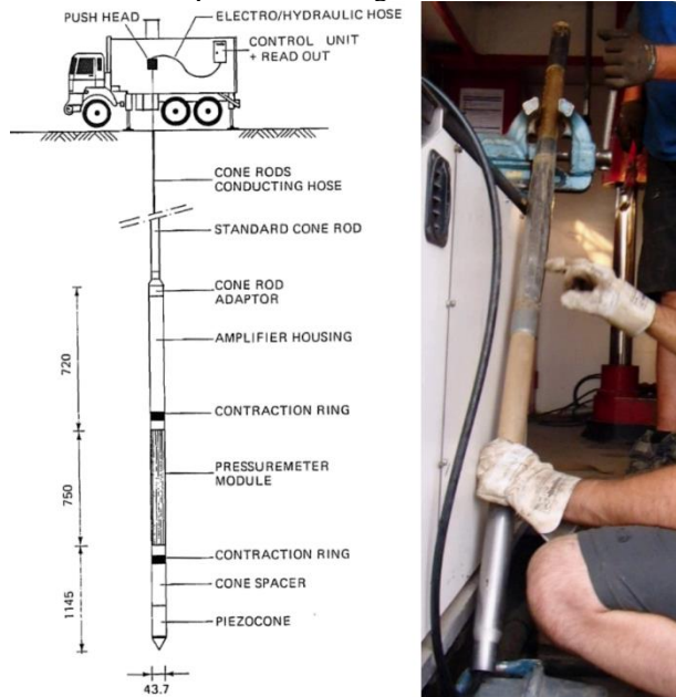
Figure 1. Left: Schematic depiction of the cone pressuremeter from Nutt (1993), and right: photo of the integrated CPM (from Cambridge Insitu / Fugro)
