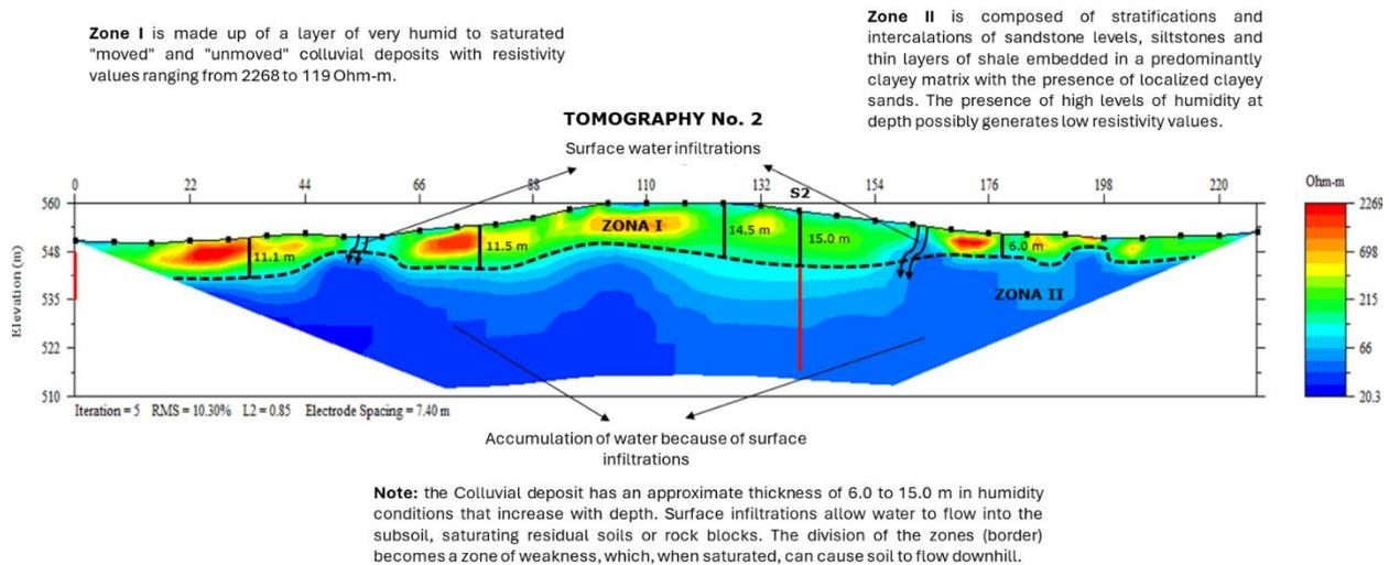
Figure 9. Example of an electrical tomography result.
