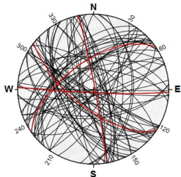
**Figure 4.** Stereographic projection of the joint planes measured in sandstones of the Diablo Formation and in mudstones and sandstones of the San Fernando Formation.
