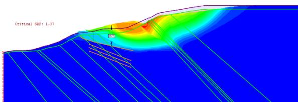
Figure 12. Result finite element stability model.
