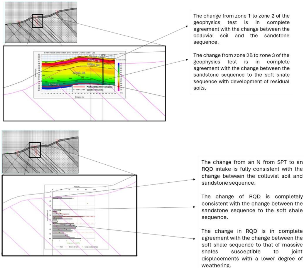
**Figure 10.** Linking of geotechnical information for verification of stratigraphy and parameters in profiles for models.
