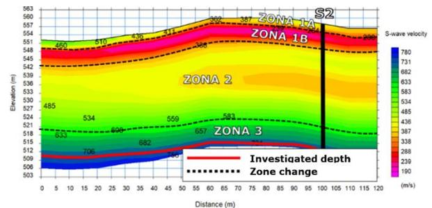
Figure 8. Example of seismic line result.
