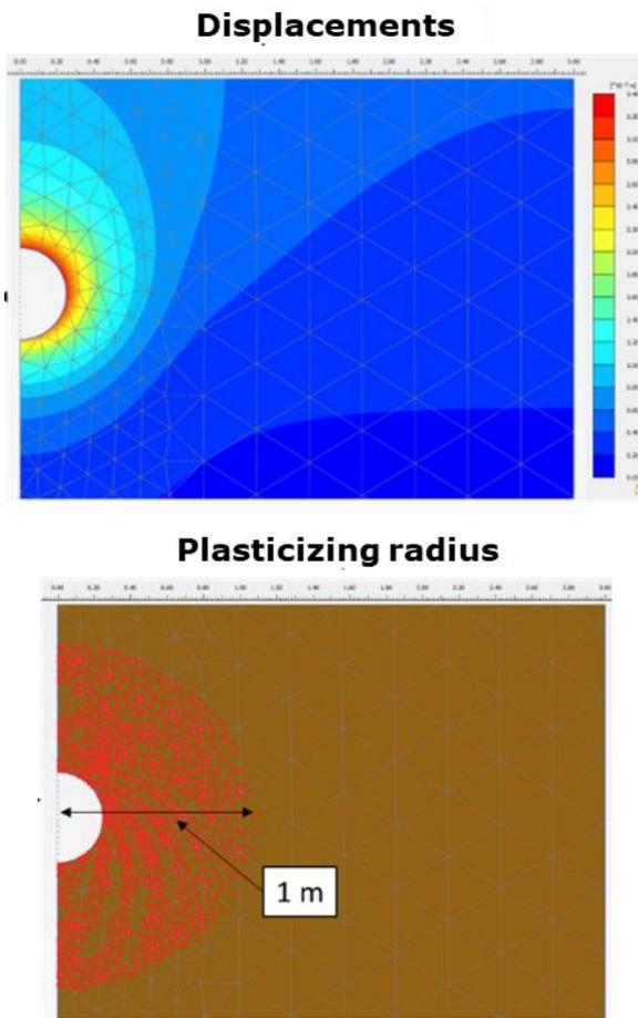
Figure 13. 2D stress-strain convergence model results.
