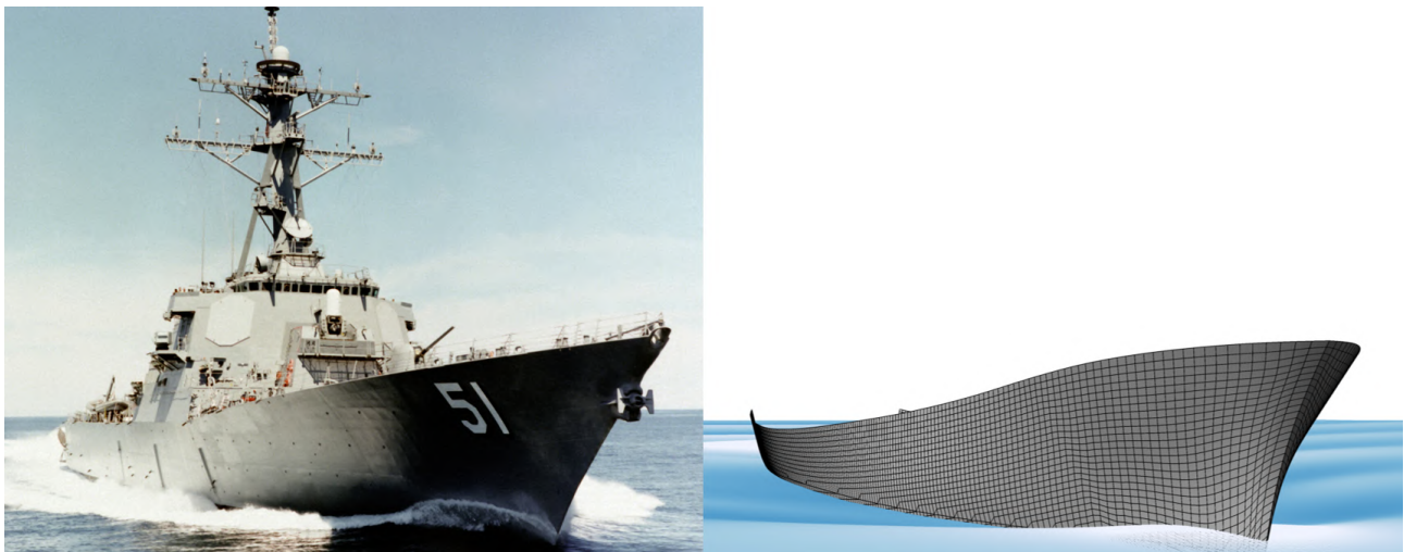
Figure 1: Starboard bow view of the guided missile destroyer Arleigh Burke (DDG-51, left) and corresponding digital counterpart of the DTMB 5415 model (right).
