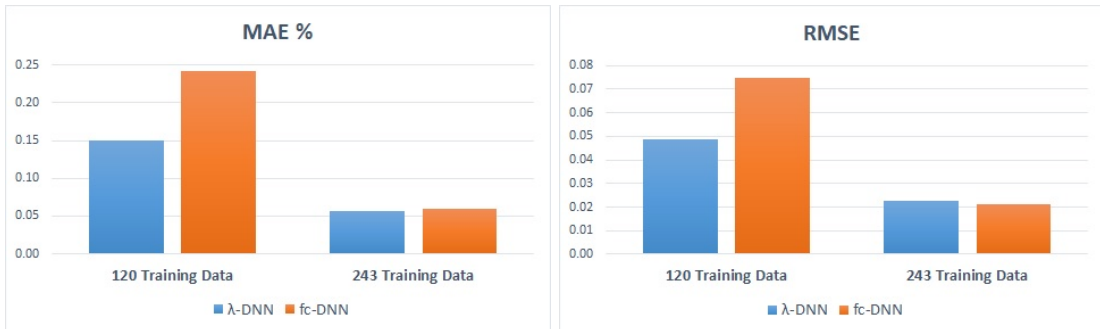
Figure 3: ONERA M6 Wing - MAE % (left) and RMSE (right) error metrics of \lambda -DNNs and fc-DNNs.
