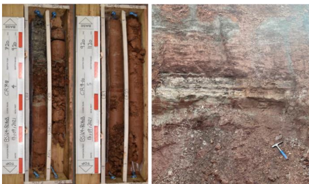
Figure 7. Left: Typical Mercia Mudstone Grade II/I borehole core example; right: Exposed geology during bulk excavation
