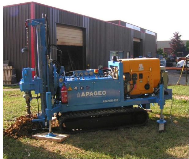
Figure 6. APAFOR 450 drilling rig.
