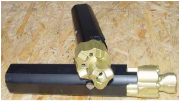
Figure 7. Blade and button eccentric drill bits (Arsonnet et al., 2005).
