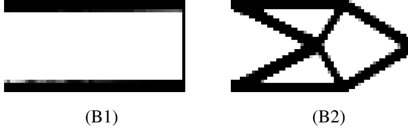
Figure 4: Density distribution of the optimized structure for benchmark cases. B1 corresponds to \mathbf{K}_c = \begin{pmatrix} 0 & 0 \\ 0 & 20 \text{ N/mm} \end{pmatrix} and B2 to \mathbf{K}_c = \begin{pmatrix} 0.01 \text{ N/mm}^{-1} & 0 \\ 0 & 0 \end{pmatrix}
