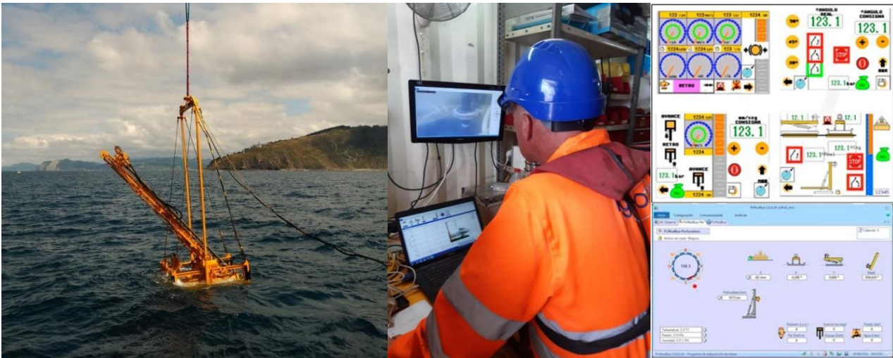
Figure 1. Submersible drilling rig (left), operator during drilling in a subsea borehole: visual inspection and drilling parameters visualisation in real time (centre) and positioning sensors for both the rig and the mast displayed (right)
