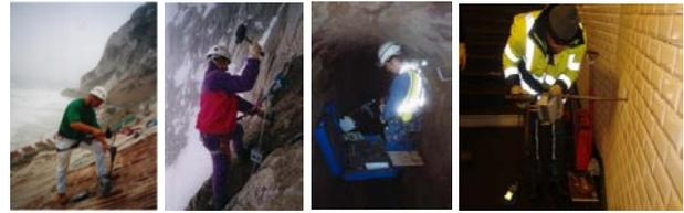
Figure 5. Examples of non-vertical penetrometric tests
