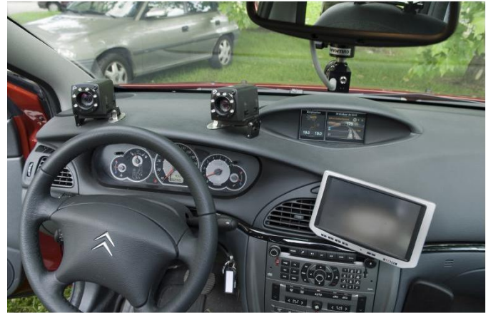
Figure 7. Driver interface: active gas pedal, audio and screen display. The two cameras on the dashboard are used for eye-tracking.
