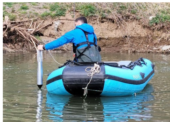
Figure 5. Portable free fall penetrometer measurements.
