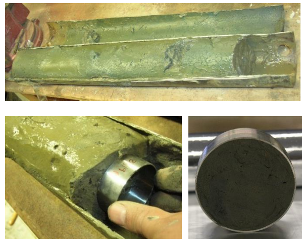
Figure 8. Cutting and sample trimming for the 88mm Shelby tube (BH1) retrieved from z = 5.5m .
