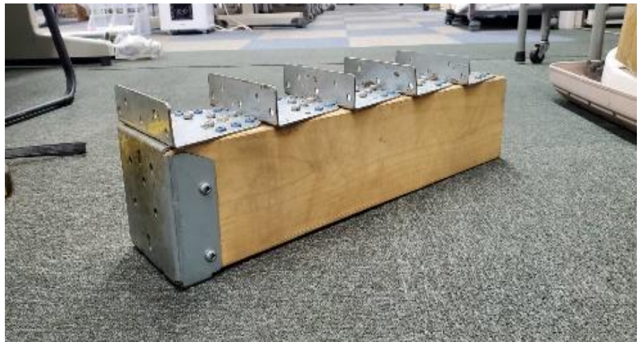
Figure. 6 Right: Artificial Vibration Exciters for SH Waves Left: Vibration excitation. Right: Structure of the exciter. A spike attached to a piece of wood is placed on the ground.
