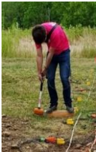
Figure. 6 Right: Artificial Vibration Exciters for SH Waves Left: Vibration excitation. Right: Structure of the exciter. A spike attached to a piece of wood is placed on the ground.
