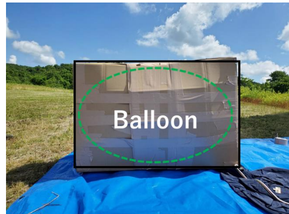
Figure. 3 The artificial cavity. The balloon is filled with air and the surrounding area is protected with reinforced cardboard.
