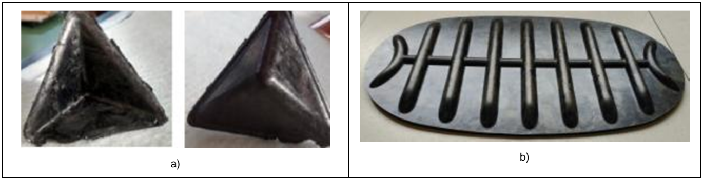
Figure 5. Aeronautical demonstrators from reused prepreg scrap, a) corner bracket, b) fuel tank access cover.
